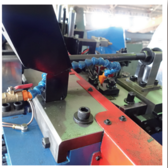
Main frame with Tie-Bar construction
